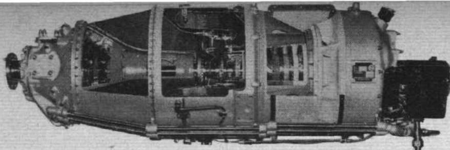
United Aircraft of Canada PT6A-20 free-turbine turboshaft. Three-stage axial plus single-stage centrifugal compressor. Annular reverse-flow combustion system. Single-stage axial h-p compressor-turbine. Single-stage axial l-p power turbine. Rating, 550 s.h.p. Weight, 275lb. Diameter, 19in
