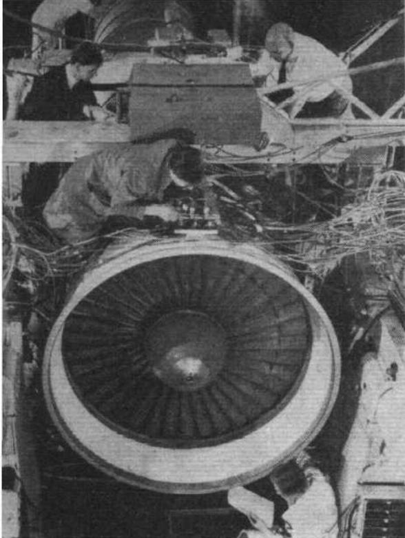
Rolls-Royce RB.178-61 twin-spool demonstrator turbofan. No design details revealed. Air mass flow, 700lb/sec. By-pass ratio, 2.75:1. Rating, 27,500lb. Diameter, 62.5in
