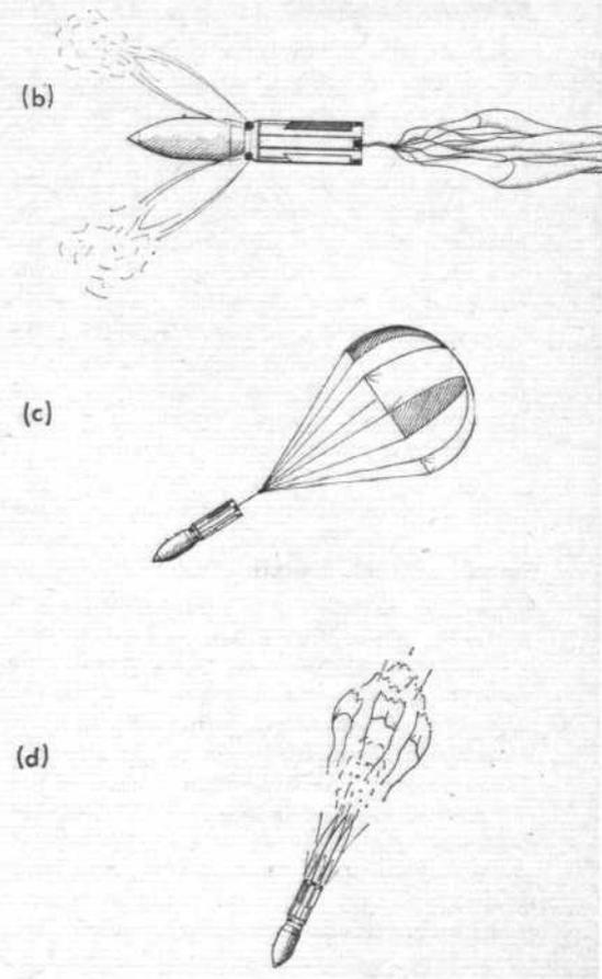
After release from an aircraft flying at only 330ft (a) the retro-rockets fire, with a time delay of 0.3sec. While they are still burning, the drogue starts deploying at 0.9sec after release. Suspended by the drogue, the bomb rotates (c) at about 20°/sec to assume its penetration angle. Then, at 4.7sec, the boosters fire and the drogue tears and burns (d)
