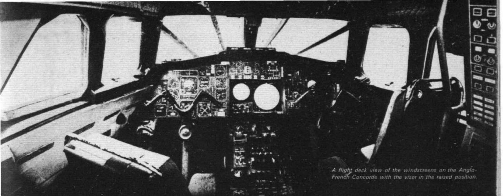
*A flight deck view of the windscreens on the Anglo-French Concorde with the visor in the raised position.*
