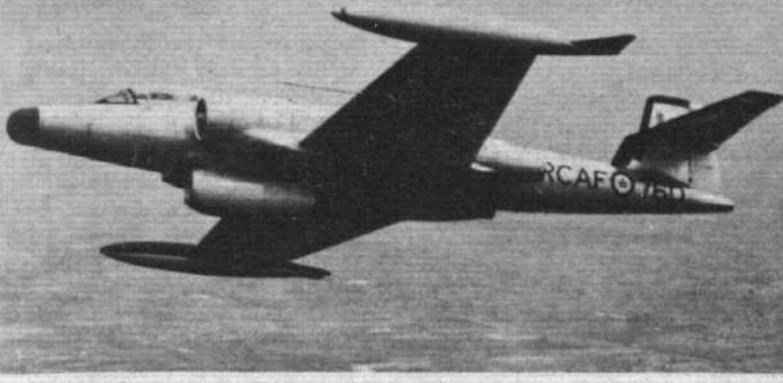
On test in an external pod slung under a CF-100 is the new United Aircraft of Canada JT15D a turbofan engine developing 2,200lb thrust. It will power the new Cessna Fanjet 500 (described on page 610) and is expected to be in production early in 1971
