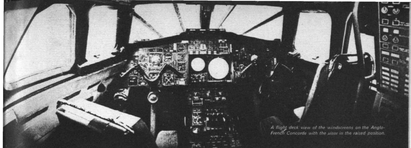
*A flight deck view of the windscreens on the Anglo-French Concorde with the visor in the raised position.*
