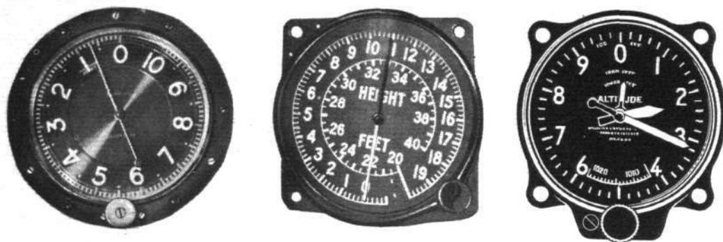
Left, one of the earliest known altimeters, vintage 1912. Centre, an instrument in use around 1930; above 20,000ft height was read off the inner scale. Right, notorious for its potential ambiguity when used in high-performance aircraft, the three-pointer altimeter was introduced in 1935 and is still in use today
