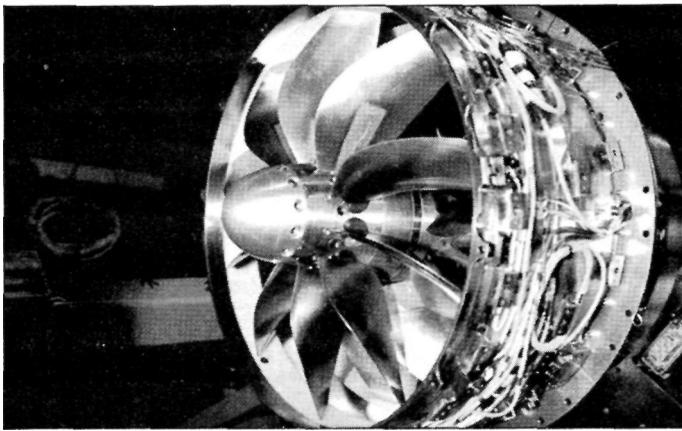
MTV's 0.4m-diameter Crisp model has two ten-blade rotors
