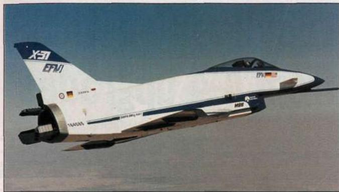
X-31 turned tail at high altitude to delude flight-control computers
