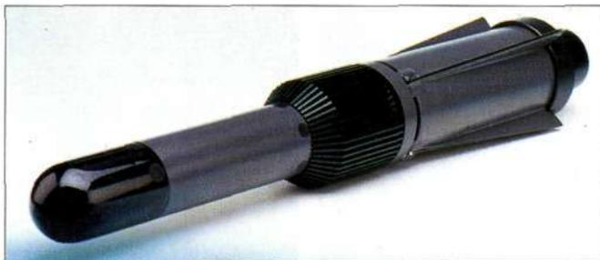
DASA's latest towed radar decoy has changed since the flight-test model
