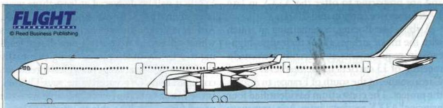
The Airbus A340-600 will have a larger wing and a new higher-thrust powerplant
