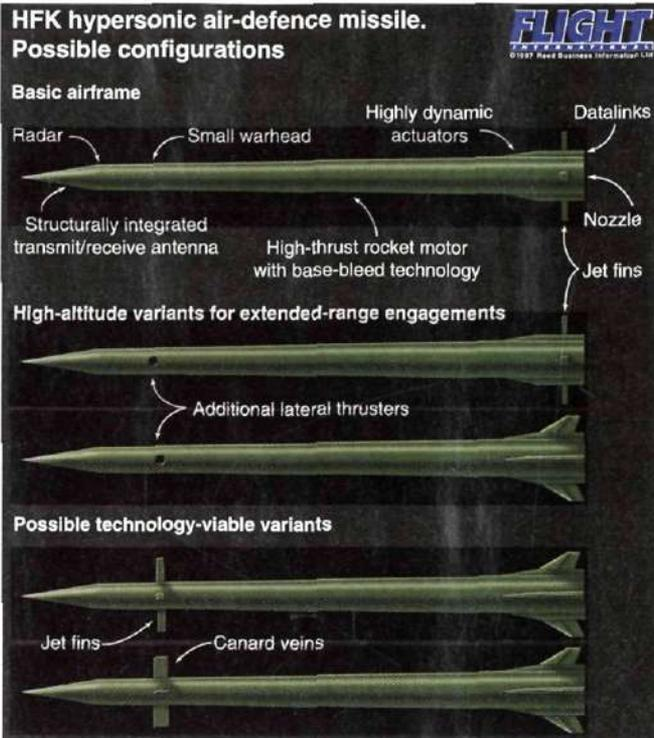
Gleich adds, however, that simulations show that hit to kill may not always be possible with a highly agile target, so the missile will carry a small explosive warhead with a proximity fuse.
