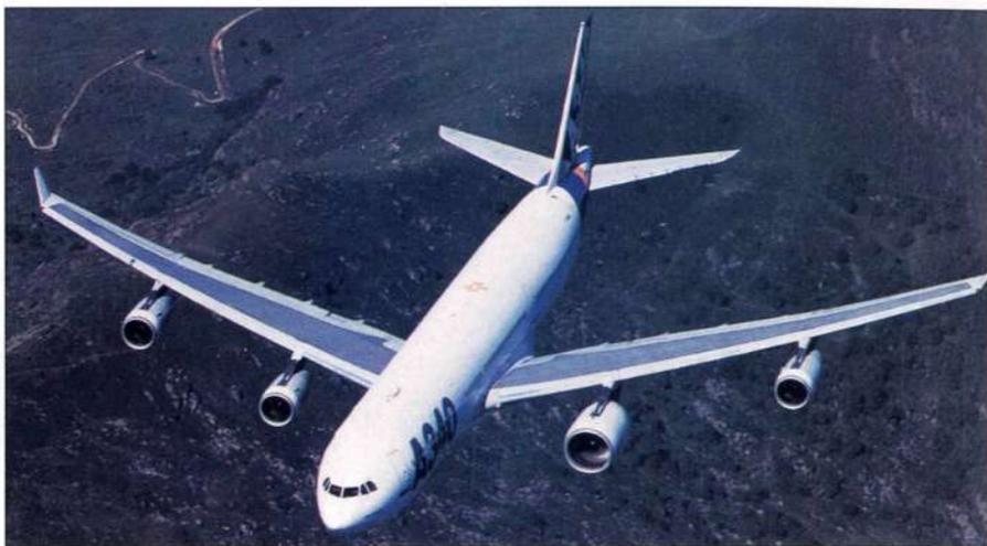
Airbus has undertaken a 47h flight-test programme of the Trent 500 on its A340-300 prototype
