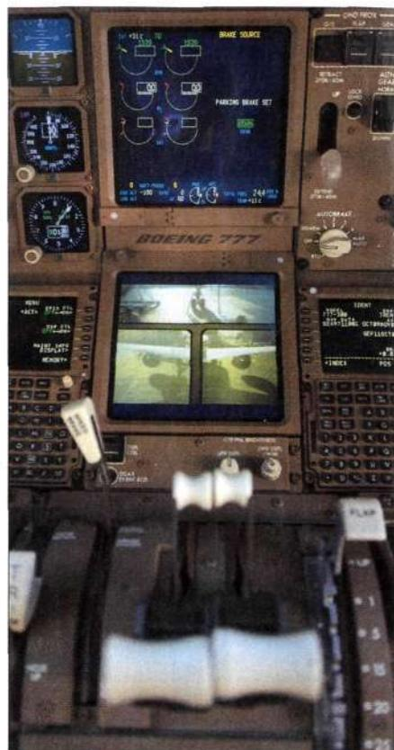
External video cameras (centre) linked with a GMCS display in the cabin cockpit (right) help the pilots manoeuvre the long -300 on the ground
