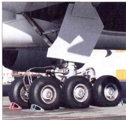
R-R Trent 892s powered the flight-test aircraft (top); a retractable tail skid prevents tail strikes during rotation (above left); all 777 versions are equipped with six-wheeled main landing gear
