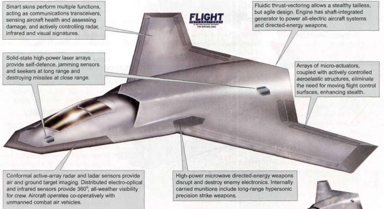
Smart skins perform multiple functions, acting as communications transceivers, sensing aircraft health and assessing damage, and actively controlling radar, infrared and visual signatures.
