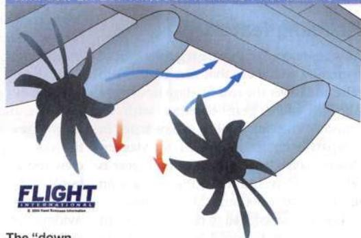
The "down between engine" innovation produces symmetric airflow, improving lift and stability
