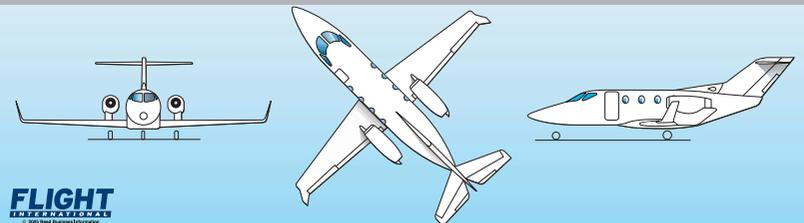
The Honda is obvious on the ramp because of the pod mounted engines above the wing. A T-tail and large winglets will also help to identify this jet.
