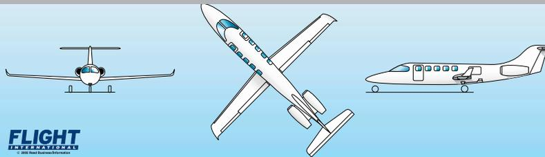
The Spectrum 33 has a T-tail and rear pod mounted engines. The wings have a high aspect ratio (the aspect ratio refers to the total span of a wing divided by the mean chord – where the chord is the length from the leading edge to the trailing edge) un-swept wing with winglets. Essentially high aspect ratio wings tend to be long and narrow, and low aspect ratios short and stubby. The 33 features five windows on each side and the cabin door is on the port side.
