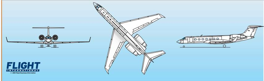
This aircraft differs externally from the legacy Gulfstream V by a seventh passenger window on the left side of the aircraft (as opposed to six on the left and either six or seven on the right). It features a low swept wing with winglets, twin Rolls-Royce Deutschland BR710 turbofan engines mounted on the fuselage ahead of a swept T-tail and swept tailplane.
