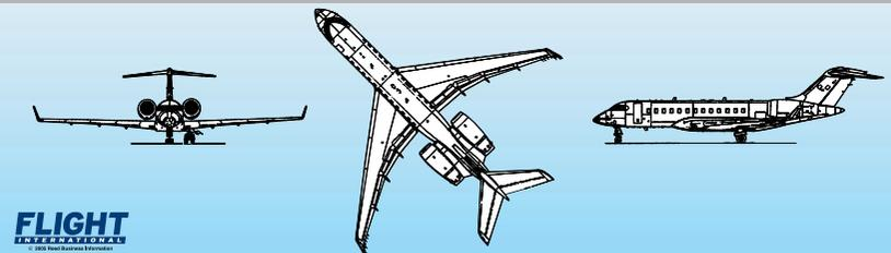
With 15 windows – Two more than the original Global Express – on each side of the cabin it clearly differentiates the XRS from the Global 5000 (with 10) and the Global Express (13). The outline of the Global Express is familiar with effectively a CRJ fuselage mated to a low swept supercritical wing with winglets. It also features a swept T-tail with swept anhedral tailplane.
