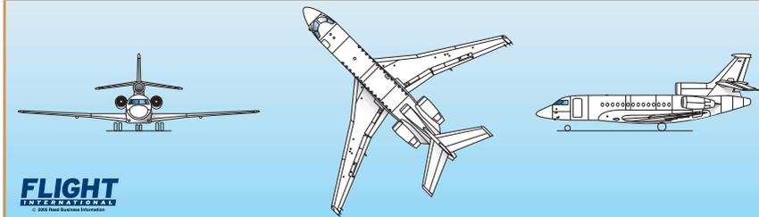
The 7X has three engines; two are pod mounted at the rear and then third is at the back of the fuselage with its air intake in front of the tail and on top of the fuselage. The wings are swept with winglets, the horizontal stabilisers are swept and mid-mounted.
